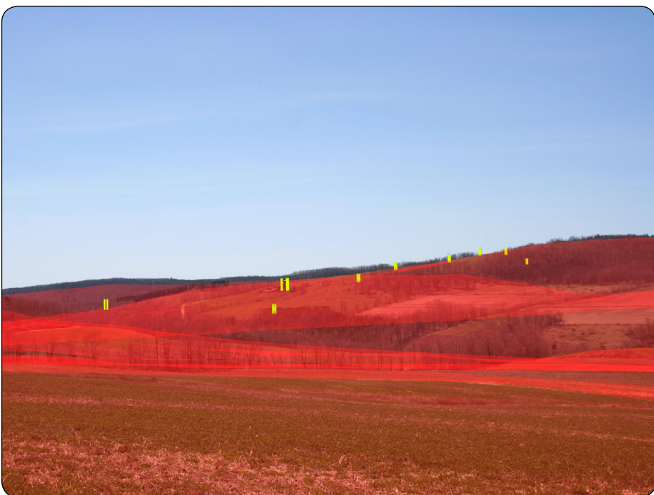
A digital terrain model representing the existing topography is also overlaid on the existing photograph to refine camera alignment, and target elevation.
