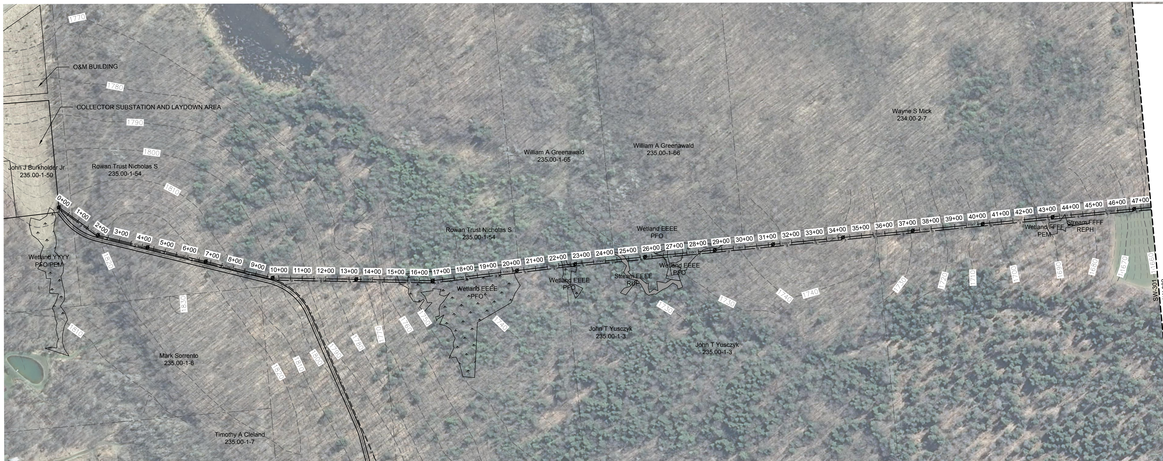
1 115 kV OVERHEAD GENERATOR LEAD LINE PLAN VIEW - STATIONS 0+00 TO 47+00 Scale: 1"=200' NOTE: POLE LOCATIONS ARE APPROXIMATE. FINAL POLE LOCATIONS, TYPE AND HEIGHT, TO BE DETERMINED BY ELECTRICAL ENGINEER.
