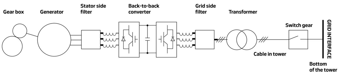
The new power system for the V112-3.0 MW<sup>®</sup> and the V126-3.0 MW<sup>™</sup> enables superior grid support. The permanent magnet generator, coupled with a full-scale converter, meets most challenging grid requirements – in almost any corner of the world.
