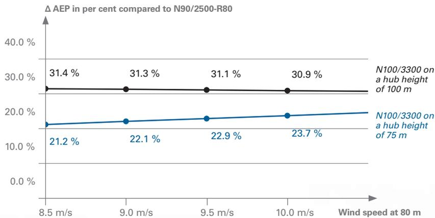
Calculation of AEP based on air density of 1.225 kg/m<sup>3</sup>, wind shear of 0.2 and Weibull shape parameter of  $k = 2.0$
